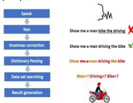
Figure 1.0 System process flow
